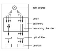
The NDIR sensor consists of a light source, optical band filters, and detectors. The light source emits a pulsing wide-band spectrum. The radiation crosses the measurement chamber. The substance being measured enters the chamber by diffusion.
